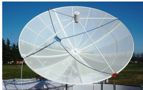
RAL10PL 11.2 GHz Total-Power Radiometer Receiver for Amateur Radio Telescope
