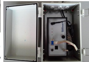
RAL10PL 11.2 GHz Total-Power Radiometer Receiver for Amateur Radio Telescope
