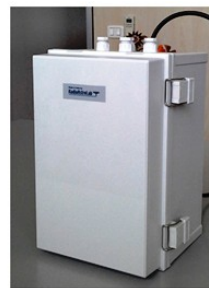
RAL10PL 11.2 GHz Total-Power Radiometer Receiver for Amateur Radio Telescope
