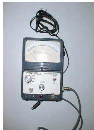
Fig. 2: Schematic of the power supply from the mains. To the right you see a prototype of the instrument. The device was built by retrieving the container (complete with moving-coil instrument) of an electronic voltmeter outside laboratory use: notice the front panel with controls for adjusting the gain and offset of the output signal of the constant integrator time. There are visible BNC connectors for signal input and output, the cable to connect the PC serial.
