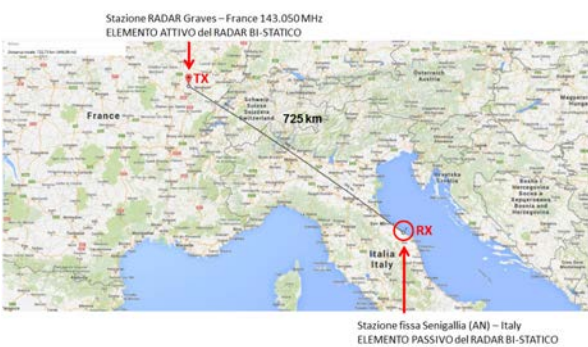
Figure 4: Distance TX-RX of the bi-static radar.
