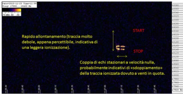
Figura 12: Multiple and complex setup of a ionized track, similar to those seen previously, with very weak vertical section and separation of the intense stationary ionization probably due to winds aloft.
