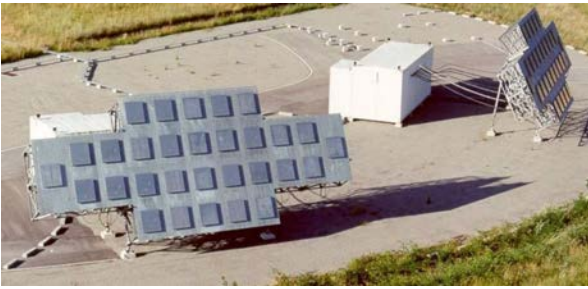
Figure 3: Two of the four panel antennas of the radar transmitter GRAVES operating at 143.050 MHz (Observatoire de Paris, Division Surveillance Espace).
