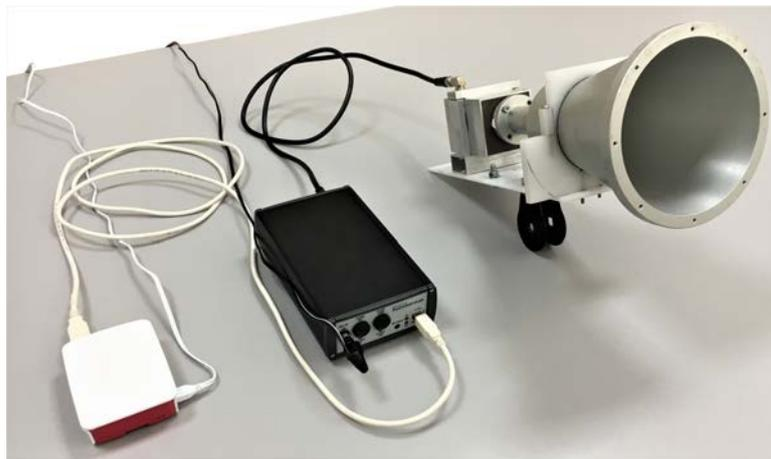
FIGURE 2.17: Working *Raspberry PI 3* with the *RAL10AP* receiver.
