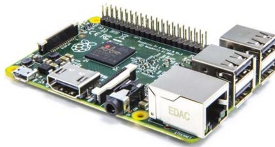
FIGURE 2.14: *Raspberry PI 3* board.
